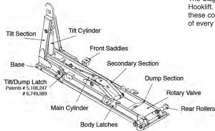
The diagram shows a typical Stellar Shuttle Hooklift. Below is a detailed explanation of these components which are an integral part of every Stellar hydraulic hooklift.
